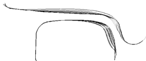
Fig. 1 Wheel wear and rail wear [8]
