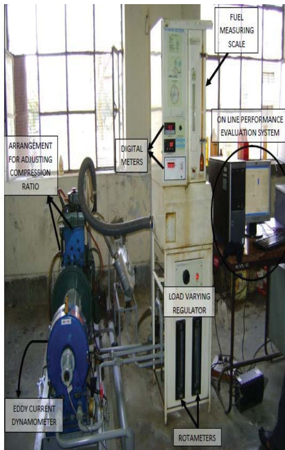
Fig. 1 Pictorial view of a single cylinder engine setup
