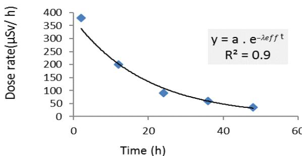
Fig.1 Exponential curve of patient external dose rate. The curve is used for calculating the effective decay constant ( $\lambda_{\text{eff}}$ )
