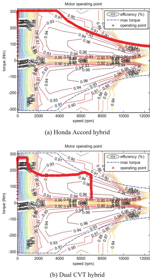
Fig. 6 Motor operating points of two hybrid systems
