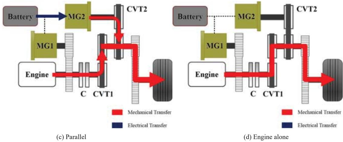
Fig. 3 Operation modes of Dual CVT hybrid system
