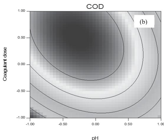
Fig. 2 Contour plots for (a) concentration, (b) COD
