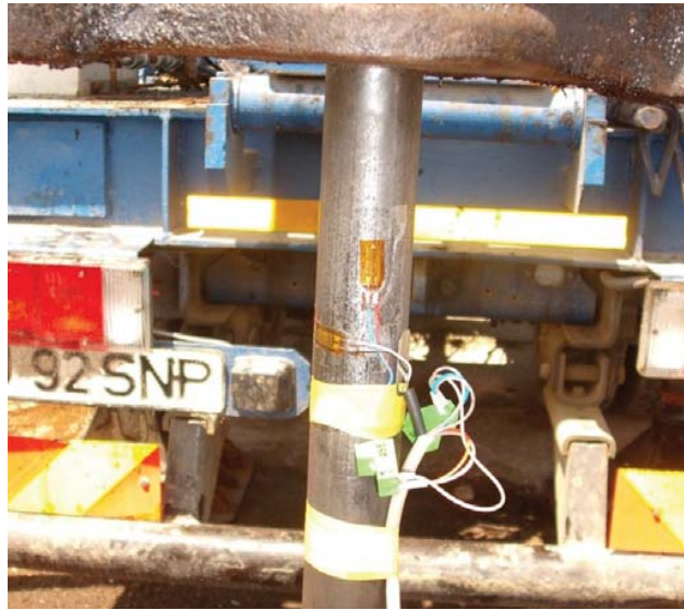
Fig. 6 Accelerometer sensor placed on the oil pumping unit polished rod
