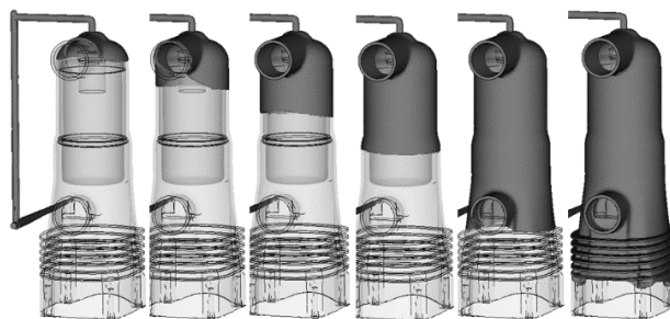
Fig. 8 Mold filling patterns during injection molding
