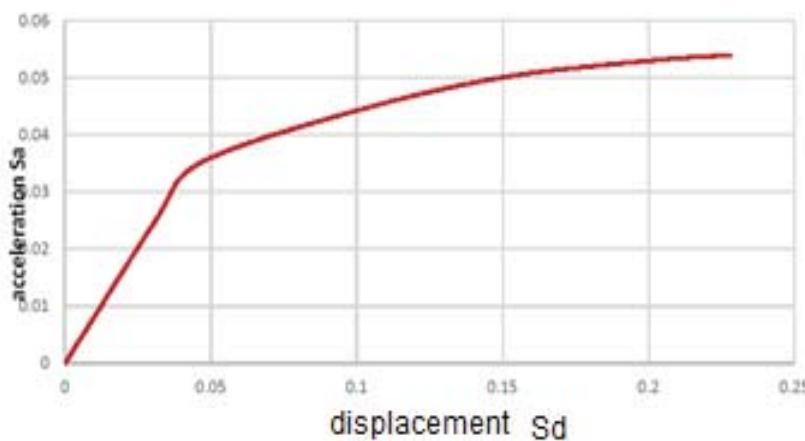
Fig. 3 Capacity spectrum of the structure (building-tank)
