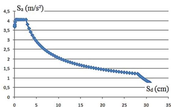
Fig. 7 Elastic response spectrum in the format ( $S_a - S_d$ )
