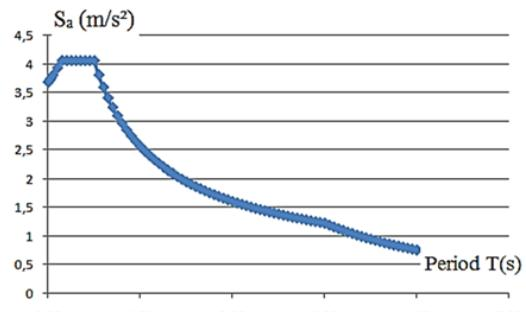
Fig. 6 Elastic response spectrum in the traditional format ( $S_a-T$ )
