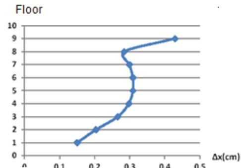
Fig. 10 Displacements between floors
