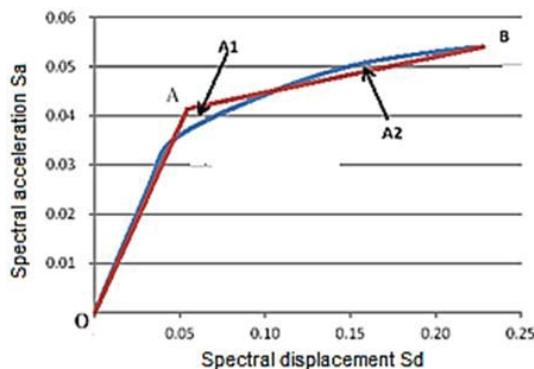
Fig. 4 Bilinear representation of the structure capacity spectrum
