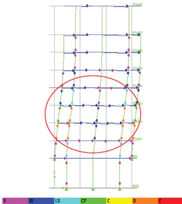
Fig. 11 Appearance of hinges of type D in the central core
