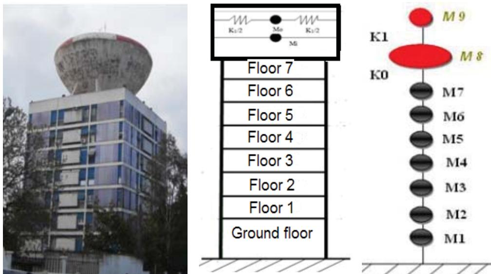
Fig. 2 Building-tank, mechanical system and mathematical model
