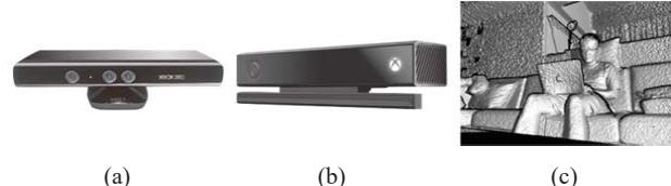
Fig. 1 (a) First generation Kinect-Kinect360, (b) second generation Kinect-Kinect V2, (c) depth information obtained by Kinect V2
