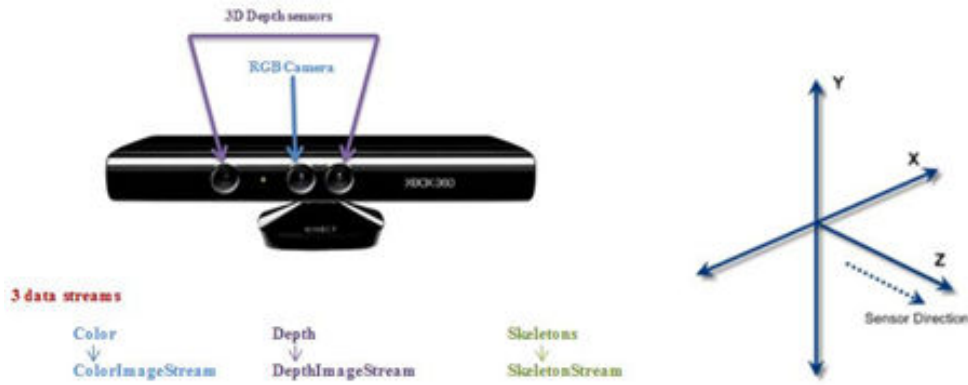
Fig. 2 Kinect Sensor and coordinate system
