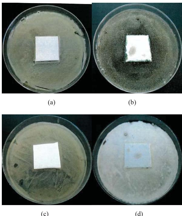
Fig. 4 Antifungal activity of zinc loaded samples: (a) *C. albicans*; (b) *A. niger*; (c) *A. pullulans* and (d) *P. chrysogenum*
