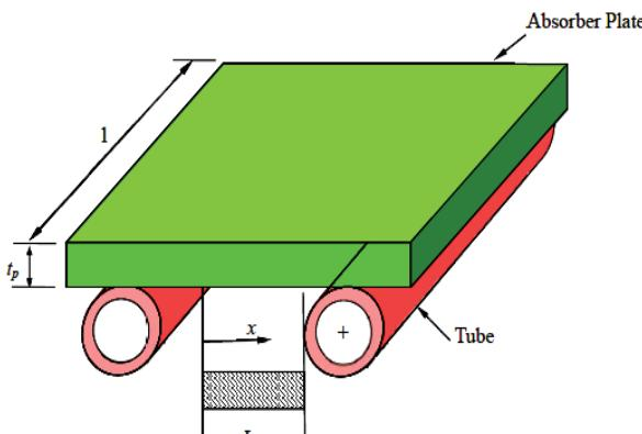
Fig. 1 Schematic of a symmetric heat transfer module in an absorber plate
