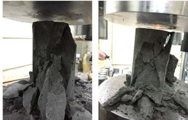
Fig. 5 Fracture aspect of 7 days compressive strength
