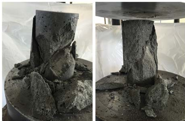
Fig. 6 Fracture aspect of 28 days compressive strength
