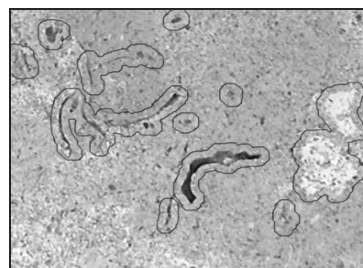
Fig. 6 Initial image with linear and spot-like, dark and clear defects localized by the methodology presented.
