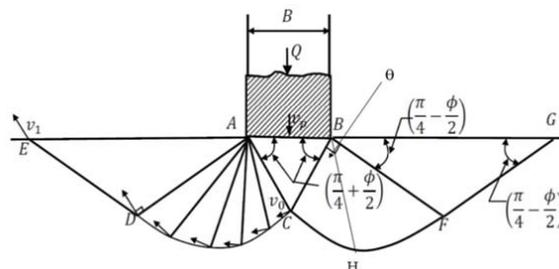
Fig. 1 Prandtl Mechanism
