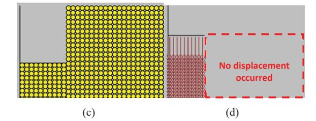
Fig. 6 Punching shear failure (contact bond=0,  $\phi=35^\circ$ , loose) (a) Model under uniform loading, (b) Displacement vectors of punching shear failure (c) Close-up view for punching shear failure and (d) Close-up view of punching shear failure
