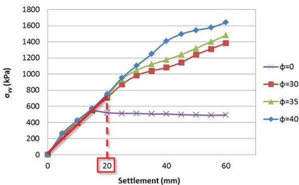
Fig. 5 Variation of vertical stress with different settlement
