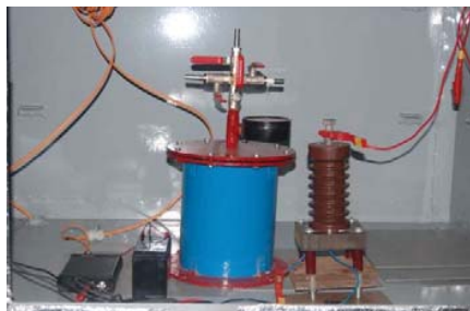
Fig. 2 High pressure test chamber
