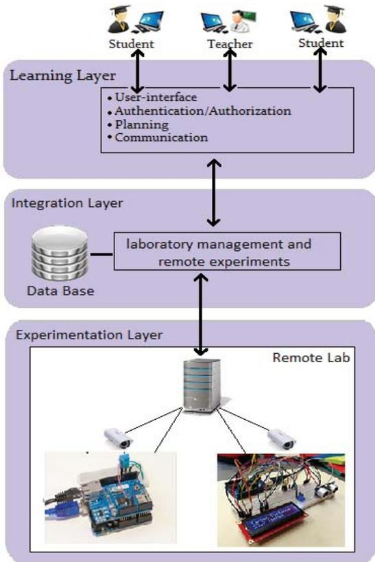
Fig. 3 The three-layer architecture of the remote lab
