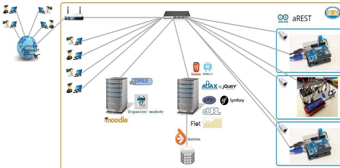
Fig. 6 Remote Lab Architecture, Technology and Tools [8]
