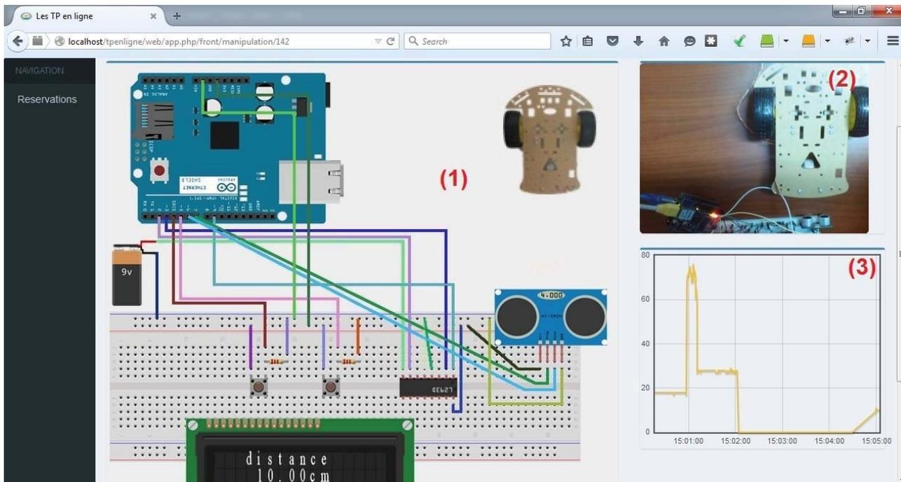
Fig. 8 The remote lab manipulation page for practical work [8]
