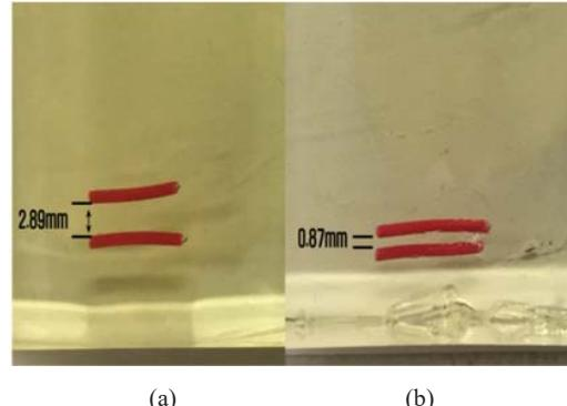
Fig. 3 The wire phantom spaced (a) 2.89mm (b) 0.87mm
