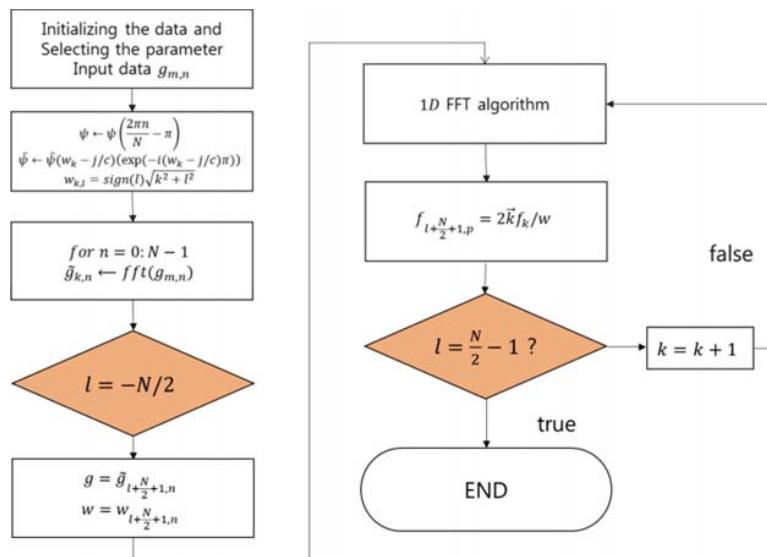
Fig. 1 Flow chart of 2D non-uniform FFT algorithm
