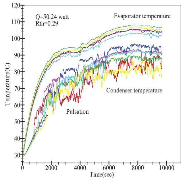
Fig. 4 Evaporator and condenser temperatures at 50.24 Watt
