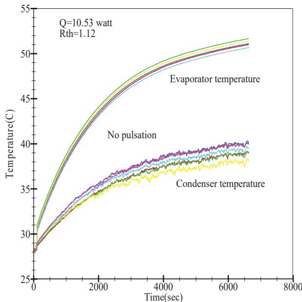
Fig. 3 Evaporator and condenser temperatures at 10.53 Watt
