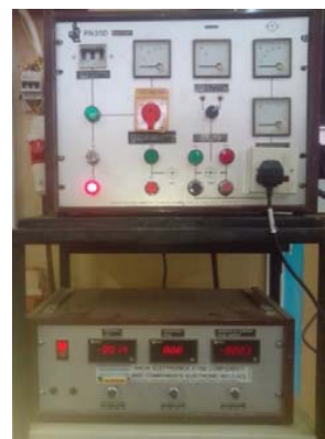
Fig. 7 Three-Component Balance Display Unit
