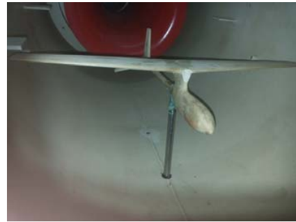
Fig. 6 Wind -Tunnel Model in Yaw Attitude
