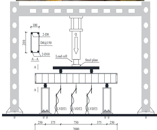
Fig. 3 Schematic if Four-Point Bending Test
