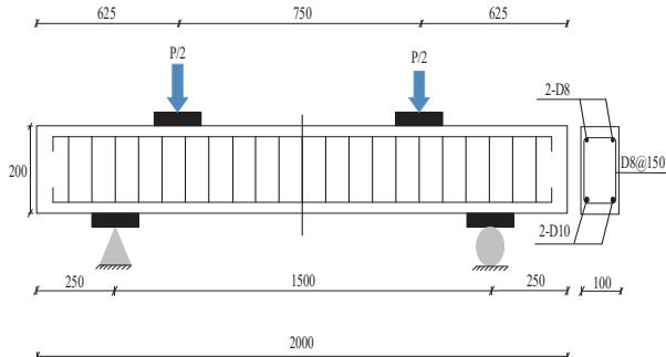
Fig. 2 Details of Geopolymer Concrete Beam
