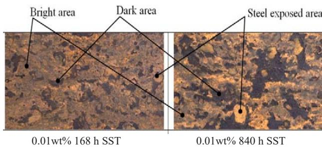
Fig. 4 Appearance of Corroded Surface after Wire Brushing
