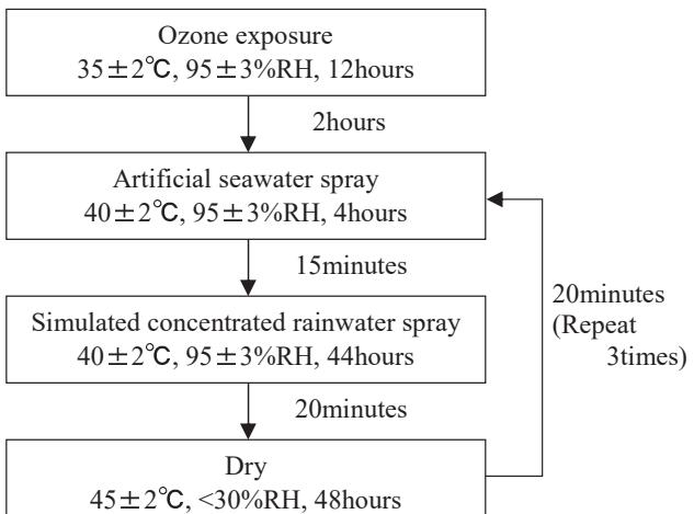
Fig. 3 Test cycle of CCT in MPASS
