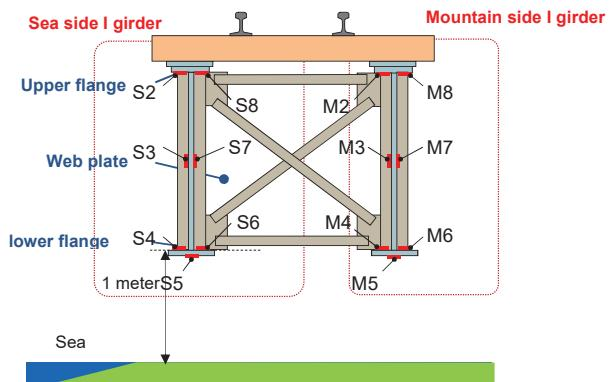
Fig. 9 Outline of the Installation Position of Each Specimen
