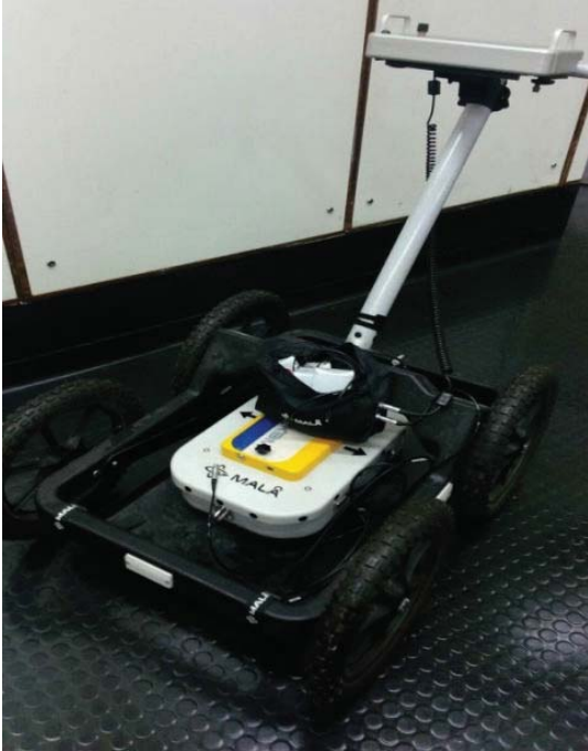
Fig. 1 GPR on a Terraplug Rough Terrain Cart
