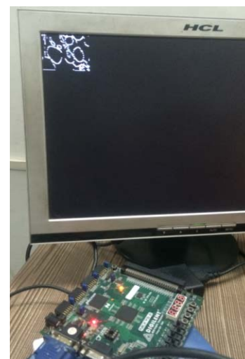
Fig. 9 VGA screen with Xilinx Vertex 4 development board
