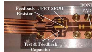
Fig. 5 Very Front End section of CC3 preamplifier designed for GERDA Phase II
