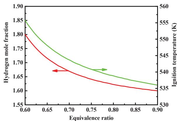
Fig. 3 Hydrogen requirement and ignition temperature versus different propane-air equivalence ratios
