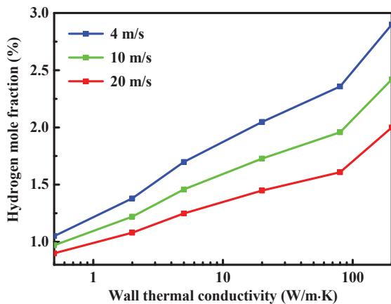
Fig. 4 Hydrogen requirement for different inlet velocities and wall thermal conductivities. The parameters used are  $\varphi$  ( $C_3H_8$ ) = 0.7 and  $h$  = 20 W/m<sup>2</sup>·K
