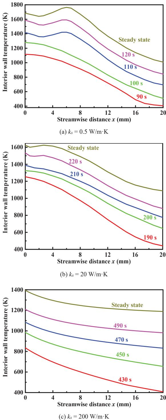
Fig. 7 Transient response of interior wall temperature profiles for various wall thermal conductivities. The parameters used are  $\phi (\text{C}_3\text{H}_8) = 0.7$ ,  $u_0 = 2 \text{ m/s}$ , and  $h = 20 \text{ W/m}^2\cdot\text{K}$
