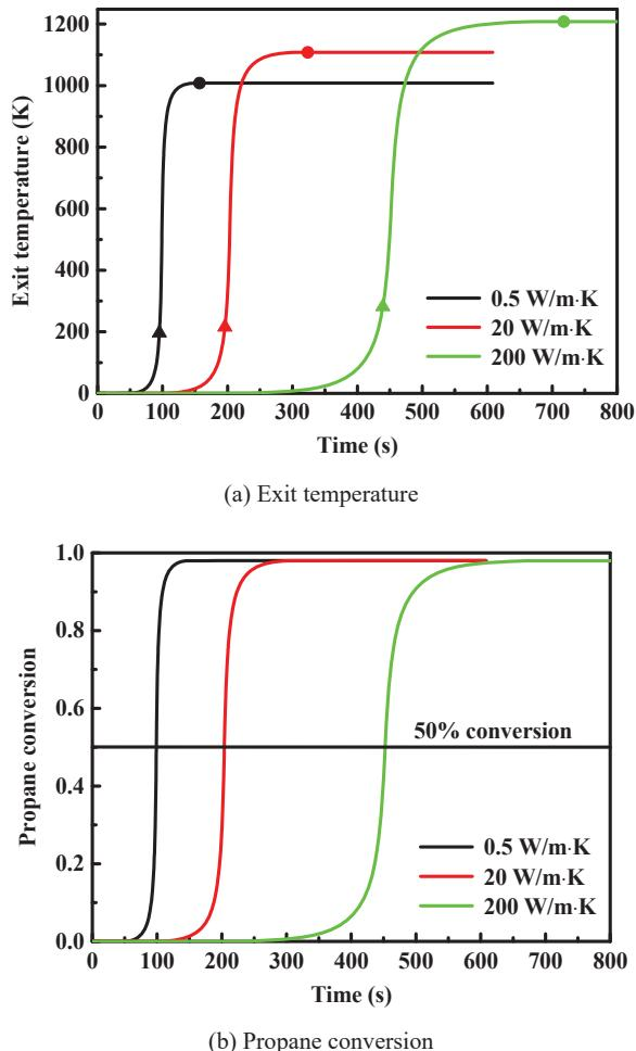
Fig. 8 Exit temperature and propane conversion profiles for different wall thermal conductivities. The parameters used are  $\phi (\text{C}_3\text{H}_8) = 0.7$ ,  $u_0 = 2 \text{ m/s}$ , and  $h = 20 \text{ W/m}^2\cdot\text{K}$ . The circles denote the steady state time  $t_{ss}$ , and the triangles denote the ignition time  $t_{ign}$ .
