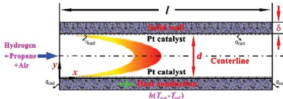
Fig. 1 Schematic diagram of the micro-channel geometry
