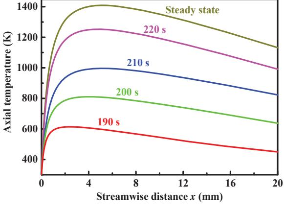
(b)  $k_s = 20 \text{ W/m}\cdot\text{K}$
