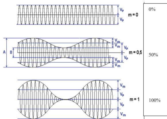
Fig. 3 Amplitude Modulation Index: 0% carrier (thermal) only, 50% (thermal and cavitational), 100% (cavitation)
