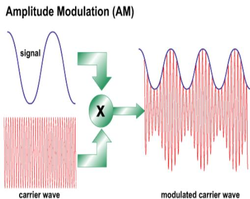
Fig. 1 Amplitude Modulation: low frequency signal modulates the amplitude of higher frequency signal (carrier)
