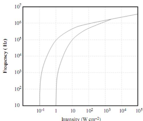
Fig. 2 Variation of intensity of sonication versus the threshold frequency: for aerated water (left-hand graph) and air-free water.
