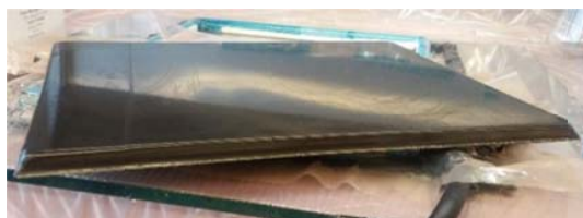
Fig. 2 Core sheets with 3% Boron Nano powder
