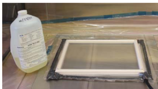
Fig. 1 Set up for preparation of core sheet
