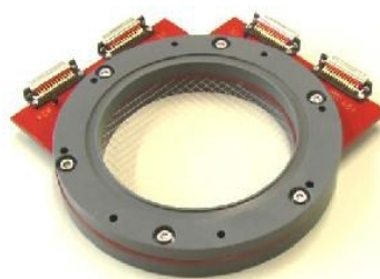
Fig. 1 Design of conductivity wire-mesh sensor
