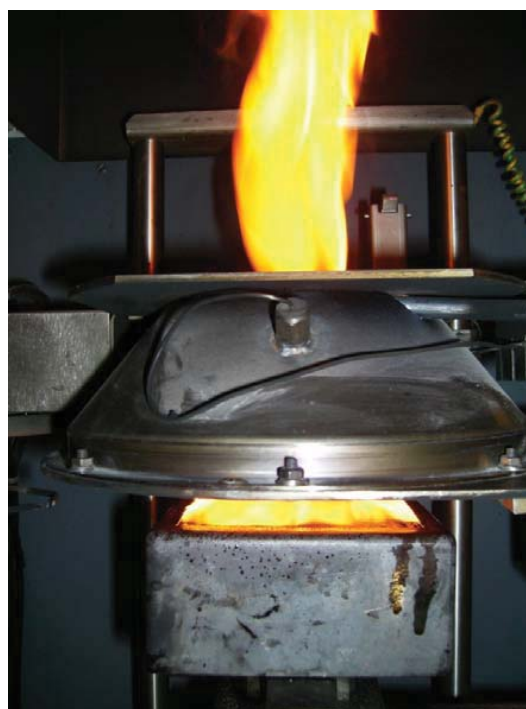
Fig. 13 Burning Latex with detail running and drops through the sample holder
