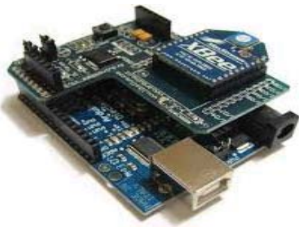
Fig. 5 Node for communication system
