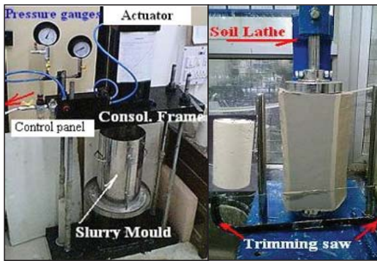
Fig. 2 Consolidation setup on the laboratory floor
