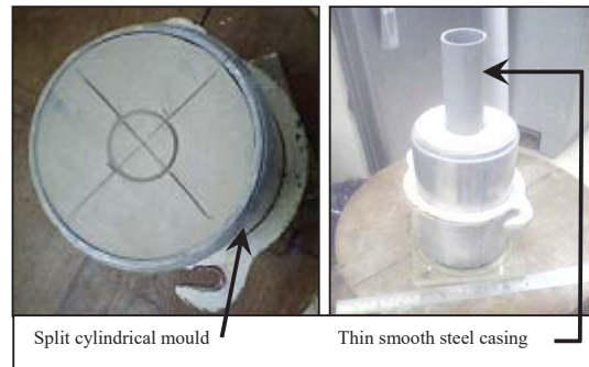
Fig. 3 Preparation of SCP in reconstituted clay specimen
