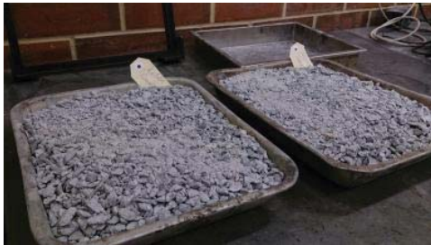
Fig. 1 Marshall Mix Design Preparations [7]
