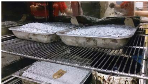
Fig. 2 Final Aggregate Mixture in Asphalt Oven [7]
