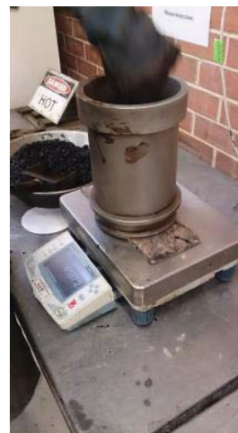
Fig. 4 Molding the Asphalt Sample [7]
