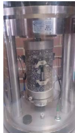
Fig. 11 Final Asphalt Specimen in AMPT [7]
