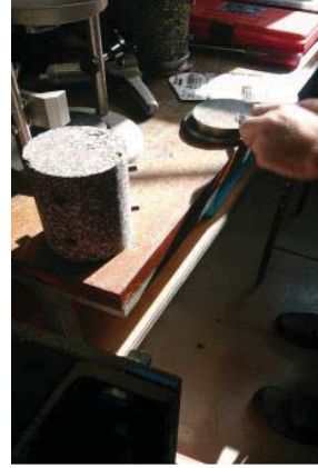
Fig. 9 Final Asphalt Specimen Underwent Gluing Process [7]
