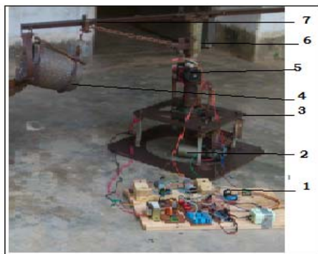
Fig. 5 Experimental models for testing robot assisted pouring systems. 1. Robot control board. 2. Motor for the rotation of robot. 3. Base frame of the robot. 4. Crucible for metal pouring. 5. Motor for crucible tilting. 6. Vertical rotating shaft. 7. Robotic arm (manipulator)
