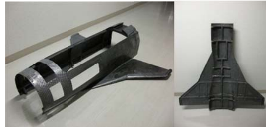
Fig. 14 Full composite semi-monocoque structure of WIRES#014
