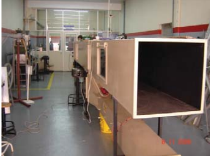
Fig. 1 Aerodynamic Air Tunnel
