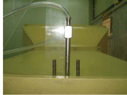
Fig. 4 Height adjustment of the Pitot tube
