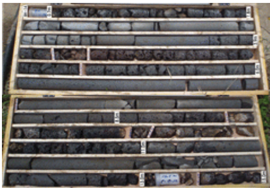
Fig. 2 Core drilling box of polymorphic ground
