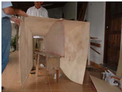
Fig. 3 Assembly of the contraction
