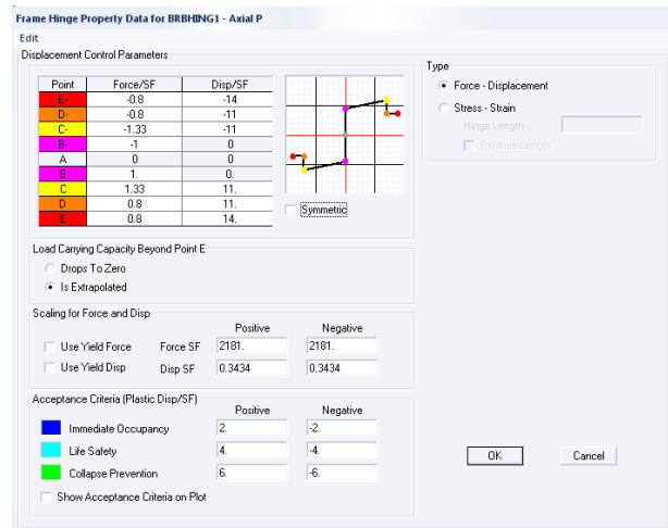
Fig. 18 The brace plastic joint of the first floor
