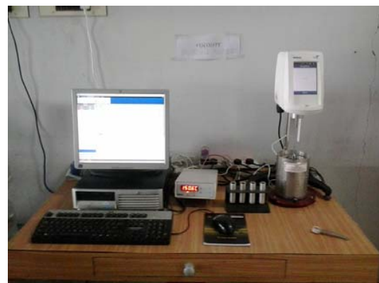
Fig. 1 Brookfield Viscometer test setup
