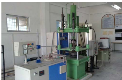
Fig. 1 Stretchforming experimentation test rig
