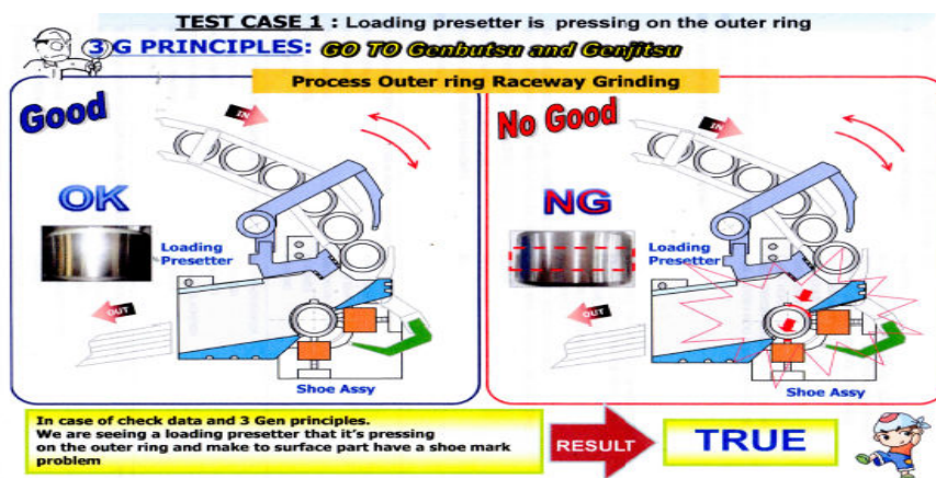
Fig. 10 Test case1: Loading presetter is pressing on the outer ring ,(persona/ 5M) [22]
