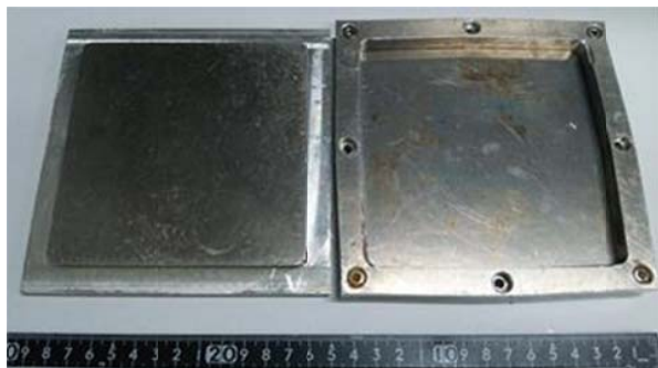
Fig. 4 Mold for vulcanizing of sheet of raw rubber materials
