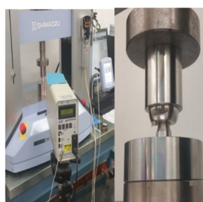
Fig. 4 Test setup of the Push-in assembly used for force application of the ball head against the stem
