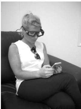
Fig. 1 The participant wearing eye tracking glasses while using iPhone 5S
