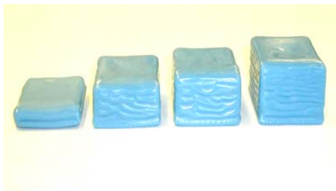
Fig. 7 Deposits of extruded wax into a square mould at 90 °C
