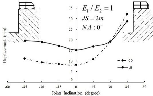
Fig. 5 Effect of joints inclination on cantilever displacement and lateral bulging, nail angle: 0°
