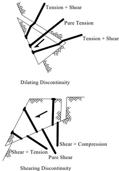
Fig. 2 Reinforcement behavior at discontinuity [2], [20]
