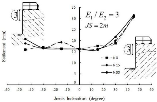
Fig. 10 Effect of joints inclination on maximum settlement where anisotropy equals to 3
