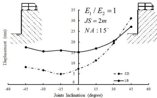
Fig. 6 Effect of joints inclination on cantilever displacement and lateral bulging, nail angle: 15°
