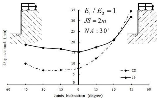
Fig. 7 Effect of joints inclination on cantilever displacement and lateral bulging, nail angle: 30°
