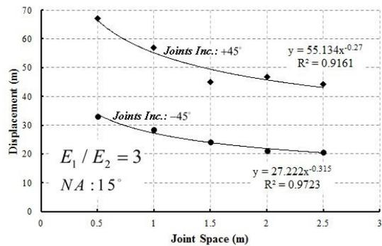
Fig. 12 Effect of joints inclination on CD
