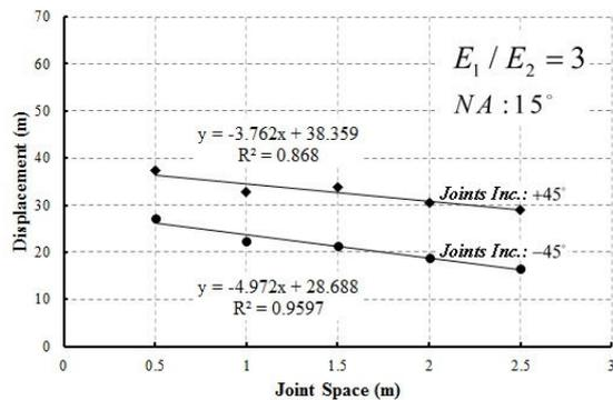
Fig. 13 Effect of joints inclination on MS
