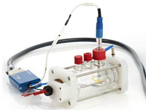
Fig. 3 Three electrode corrosion cell (capacity 300 cm 3 )
