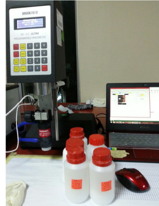
Fig. 2 Viscosity measurement using LVDV-III Brookfield rheometer
