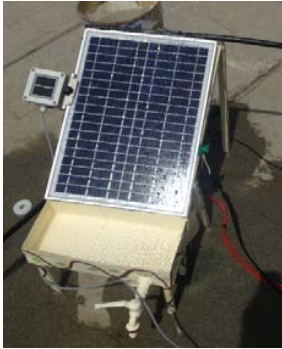
Fig. 1 PV panel and cooling system used during experiment
